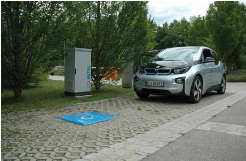
BMW i3 with wireless inductive charging retrofit, in daily use in Munich
